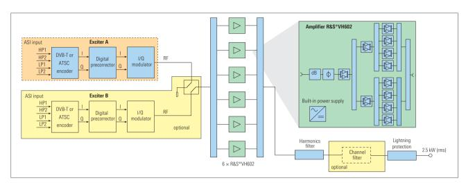
Block diagram of the 2.5 kW DVB-T transmitter or 4.1 kW ATSC transmitter
